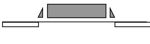
Figure 5.3. Sidewall extensions of MOSFET gate (Toshiba).
