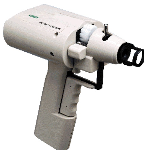
Figure 8.3. Pictured here is the “Gene Gun,” a system that uses nanoparticles to deliver genetic material to transfect plant and animal cells. In this system, submicron gold particles coated with DNA are accelerated with a supersonic expansion of helium gas. The particles leave the front of the device at high velocity and penetrate the cell membrane and nuclear membrane, thus delivering the genetic material to the nucleus (courtesy Bio-Rad Laboratories).
